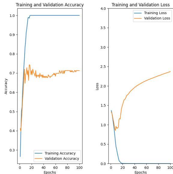
Figure 3. Basic CNN training plots corresponding to a single training run under the fixed 70/20/10 partition with no smoothing applied.
