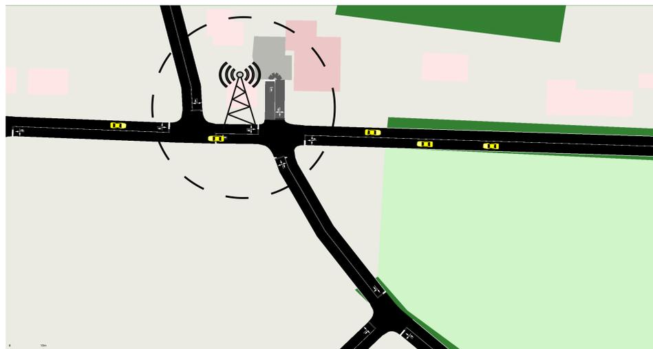
Figure 11. V2R Communication for Updating RV and obtaining Pre-Signature from RSU.
