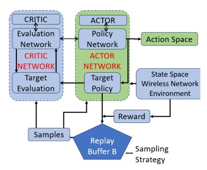
Figure 1. Abstract view of the interrelationship between DDPG-MPCC Modules.
