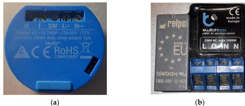
**Figure 6.** Smart home switch modules: (a) Shelly 1 and (b) Blebox Switchbox.
