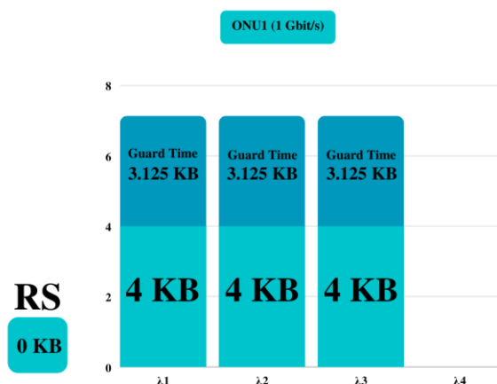
Figure 4. The allocated bandwidth of three wavelengths for the ONU1 bandwidth request with the addition of guard times.
