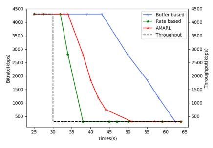
Figure 8. Variation of the bitrate of different algorithms when the throughput drops suddenly.
