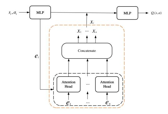
**Figure 3.** Calculating  $Q_i^{\psi}(s, a)$  for *agent<sub>i</sub>*. Each agent encodes its observations and actions, sends them to the central attention mechanism, and receives a weighted sum of other agents' encodings.
