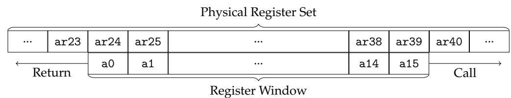
Figure 1. Example of a register window mapping of logical registers a0–a15 to physical registers ar24–ar39.
