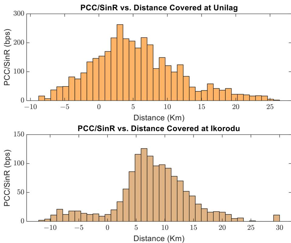
Figure 11. Histogram of the ratio of the packet component carrier (PCC) to the signal-to-noise ratio (SINR).
