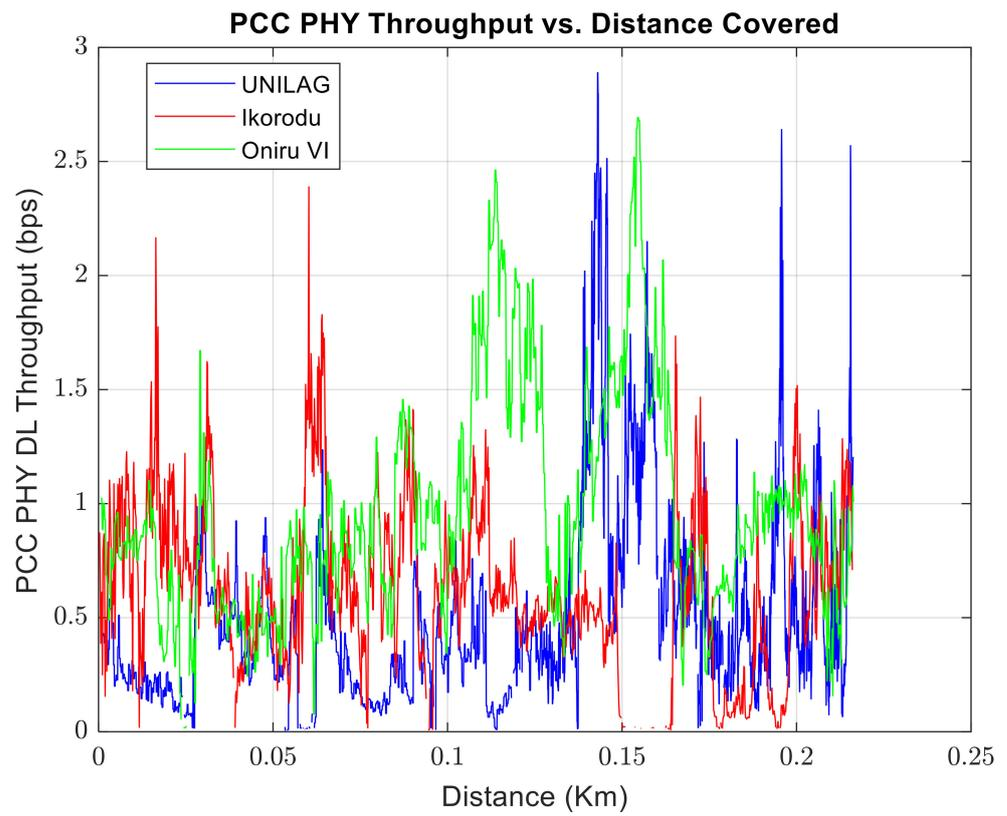
Figure 6. Signal monitoring of the packet component carrier (PCC) physical (PHY) downlink (DL) throughput.
