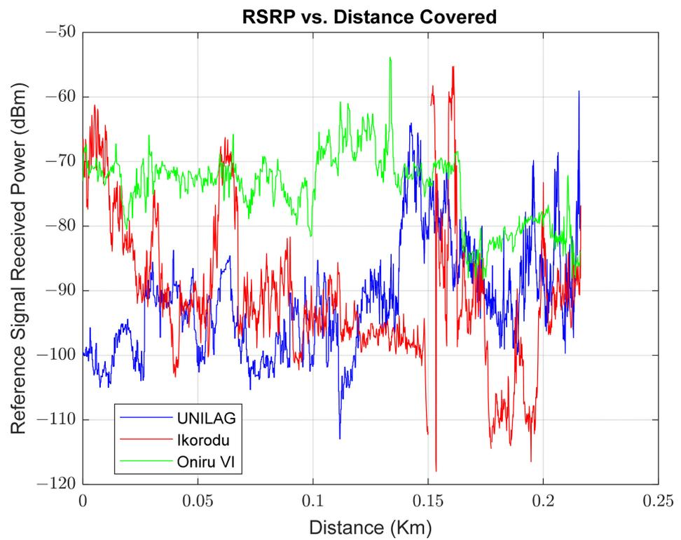
Figure 2. Signal monitoring of the reference signal received power (RSRP).
