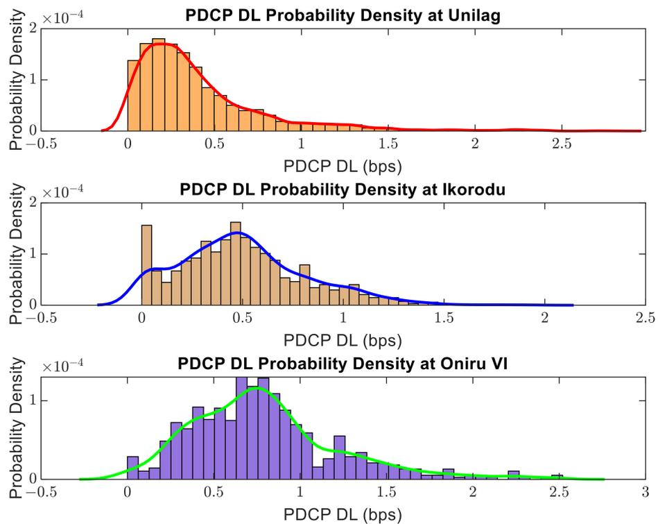
**Figure 19.** Probability density function of the packet data convergence protocol (PDCP) downlink (DL) throughput.
