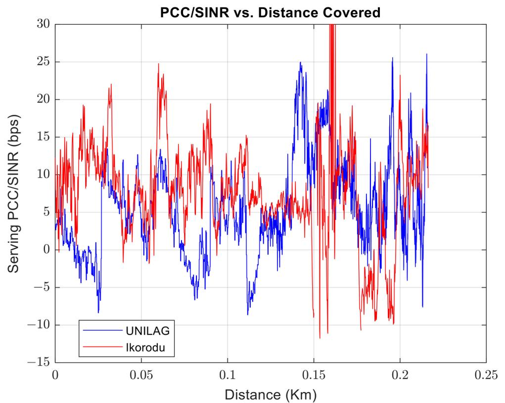
Figure 5. Signal monitoring of the ratio of the packet component carrier (PCC) to the signal-to-noise ratio (SINR).
