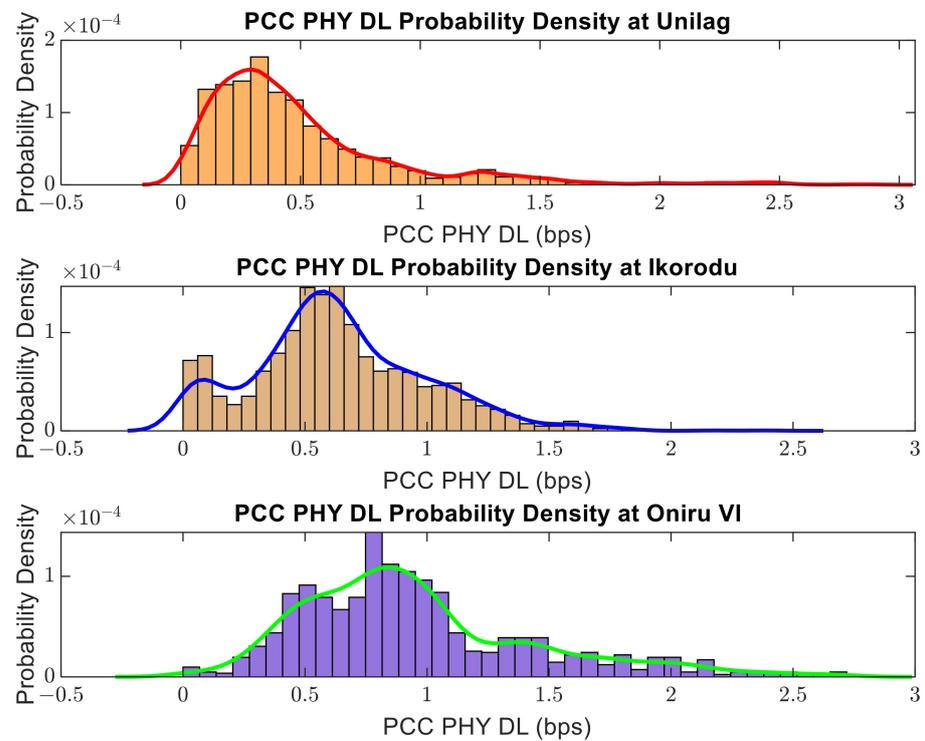
**Figure 18.** Probability density function of the packet component carrier (PCC) physical (PHY) downlink (DL) throughput.
