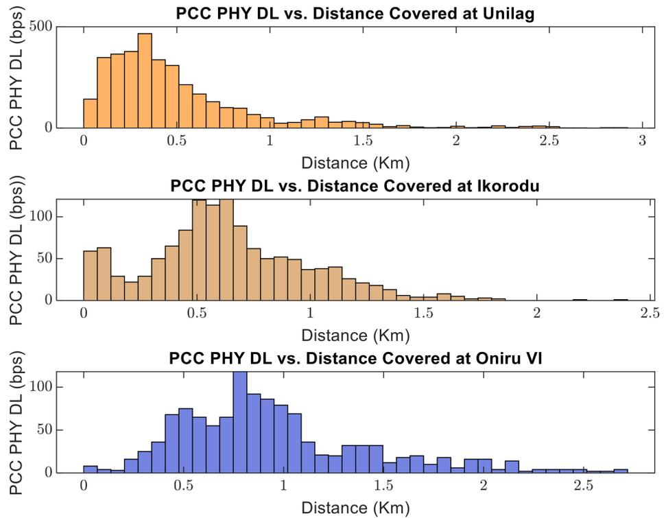
Figure 12. Histogram of packet component carrier (PCC) physical (PHY) downlink (DL) throughput.
