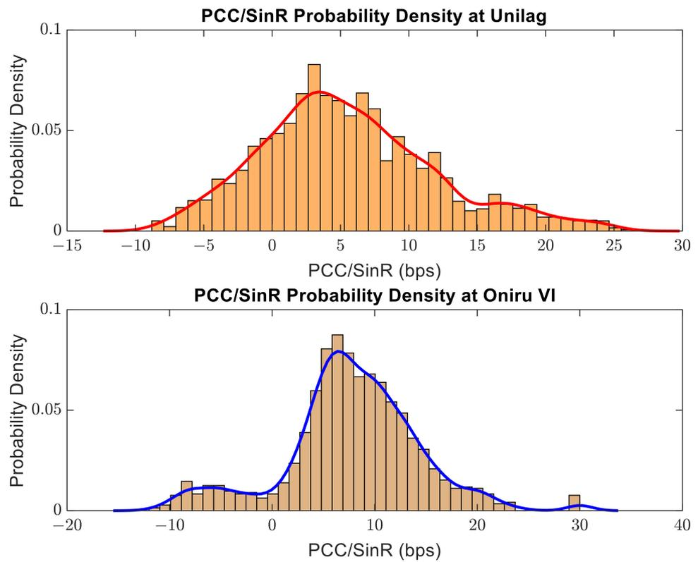
**Figure 17.** Probability density function of the ratio of the packet component carrier (PCC) to the signal-to-noise ratio (SINR).
