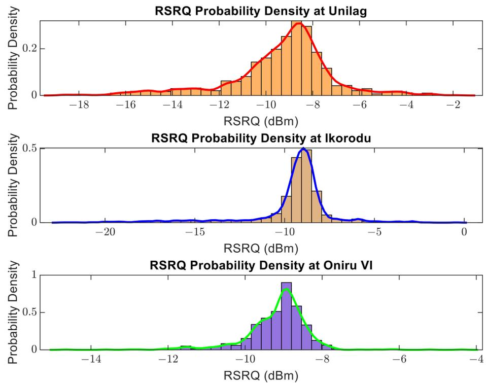
Figure 15. Probability density function of the reference signal received quality (RSRQ).
