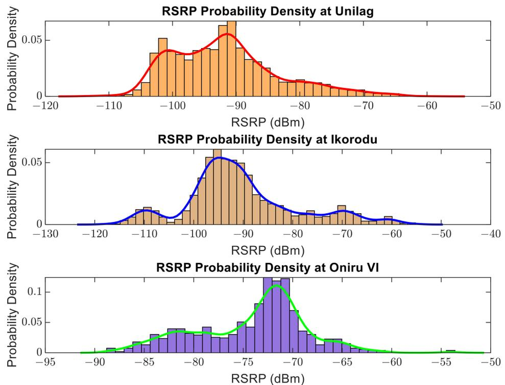
**Figure 14.** Probability density function of the reference signal received power (RSRP).
