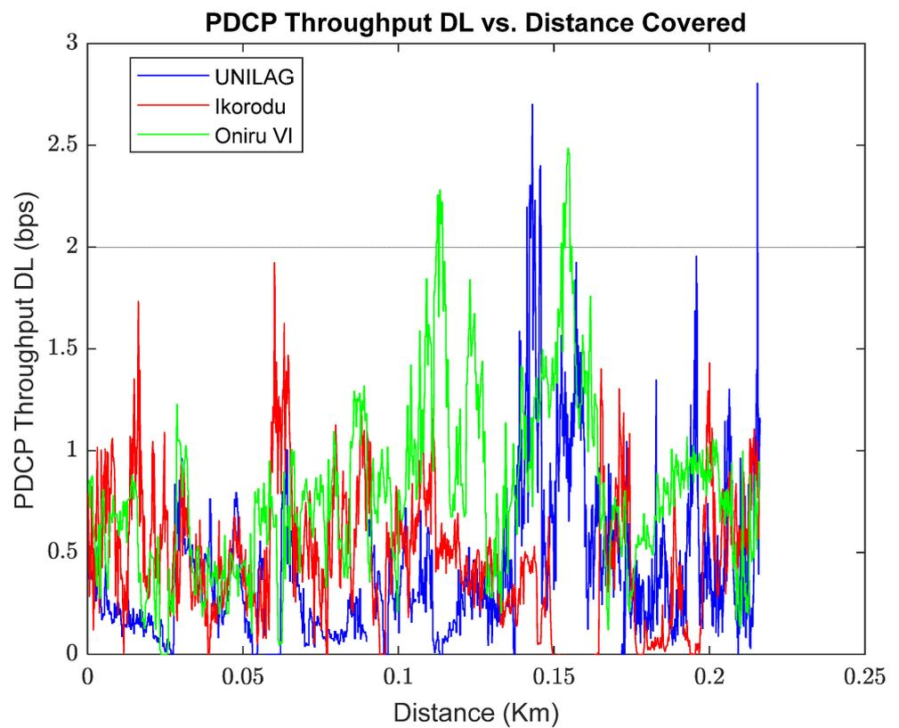
Figure 7. Signal monitoring of the packet data convergence protocol (PDCP) downlink (DL) throughput.
