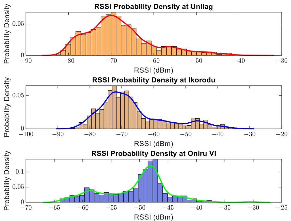
Figure 16. Probability density function of the received signal strength indicator (RSSI).
