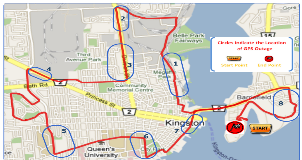
Figure 11. Road test trajectory and circles indicate the approximate locations of 120 s GNSS outages.
