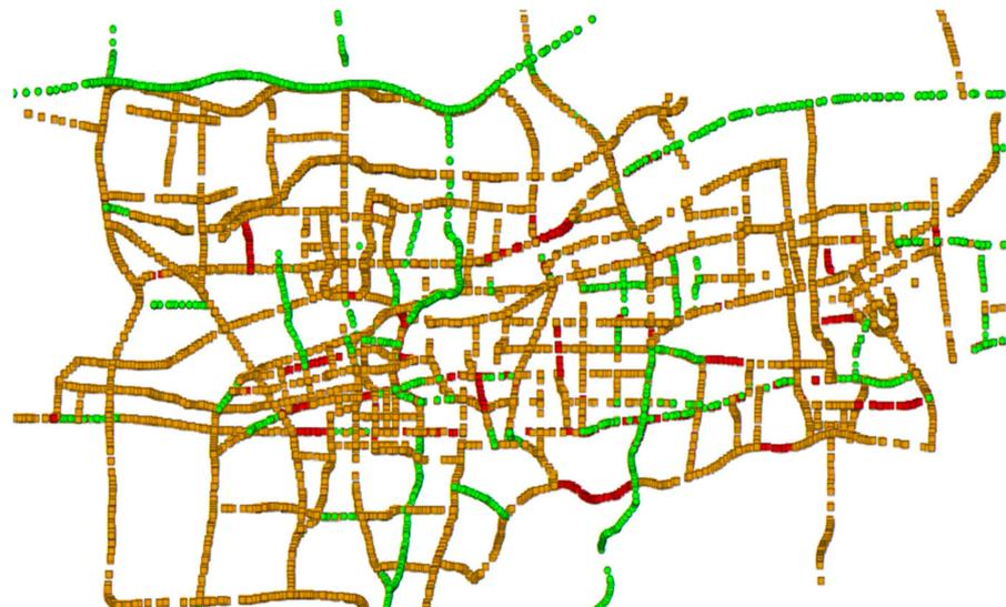
**Figure 4.** Road condition in the late morning rush hour in Jinan city. (The closer the road color is to green, the smoother the road. The closer the road color is to red, the more congested it is).
