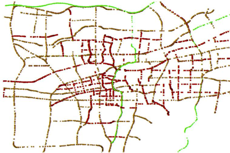
**Figure 6.** Evening rush hour road conditions. (The closer the road color is to green, the smoother the road. The closer the road color is to red, the more congested it is).
