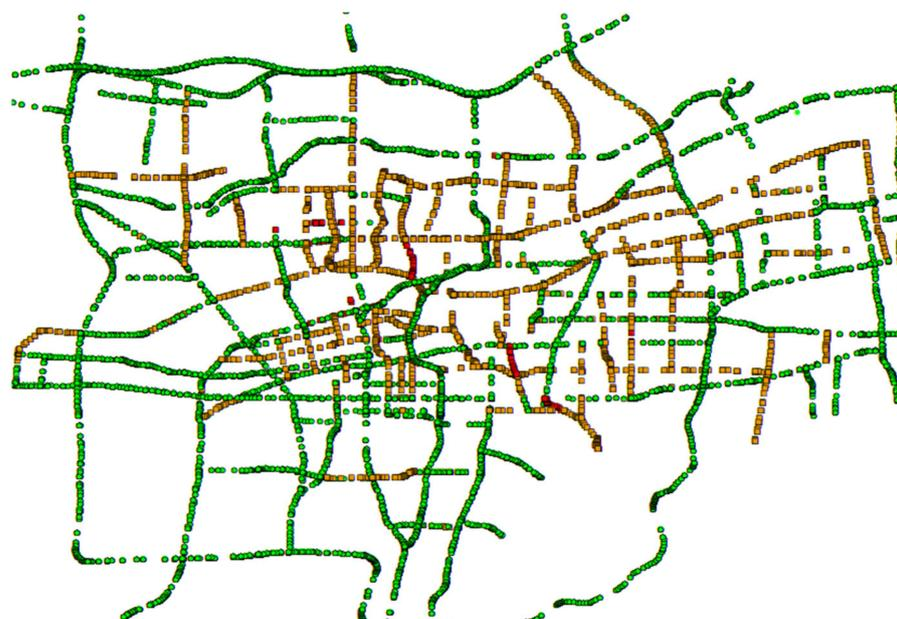
**Figure 5.** Road conditions at other times of weekdays. (The closer the road color is to green, the smoother the road. The closer the road color is to red, the more congested it is).
