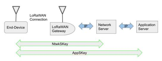
Figure 2. LoRaWAN Secure Architecture.
