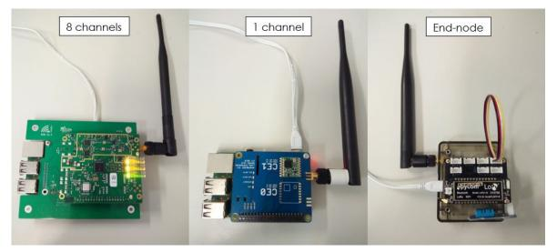
Figure 8. BS with eight channels gateway (left), BS with single channel GW (middle) and end-node (right).
