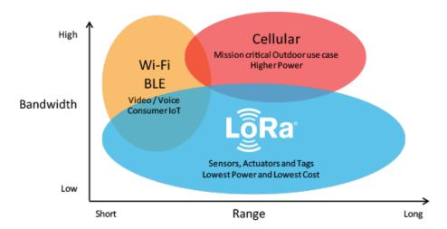
**Figure 1.** Why LoRa? LoRa has a greater power budget than Cellular or WiFi and therefore can achieve a greater range or deeper in building coverage, by using a much lower data rate.
