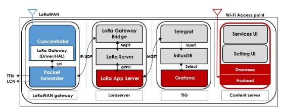
Figure 7. Four main parts of the Base Station.
