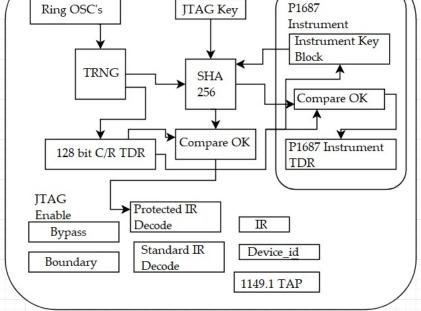
Figure 3. IC with anti-tamper JTAG [29].
