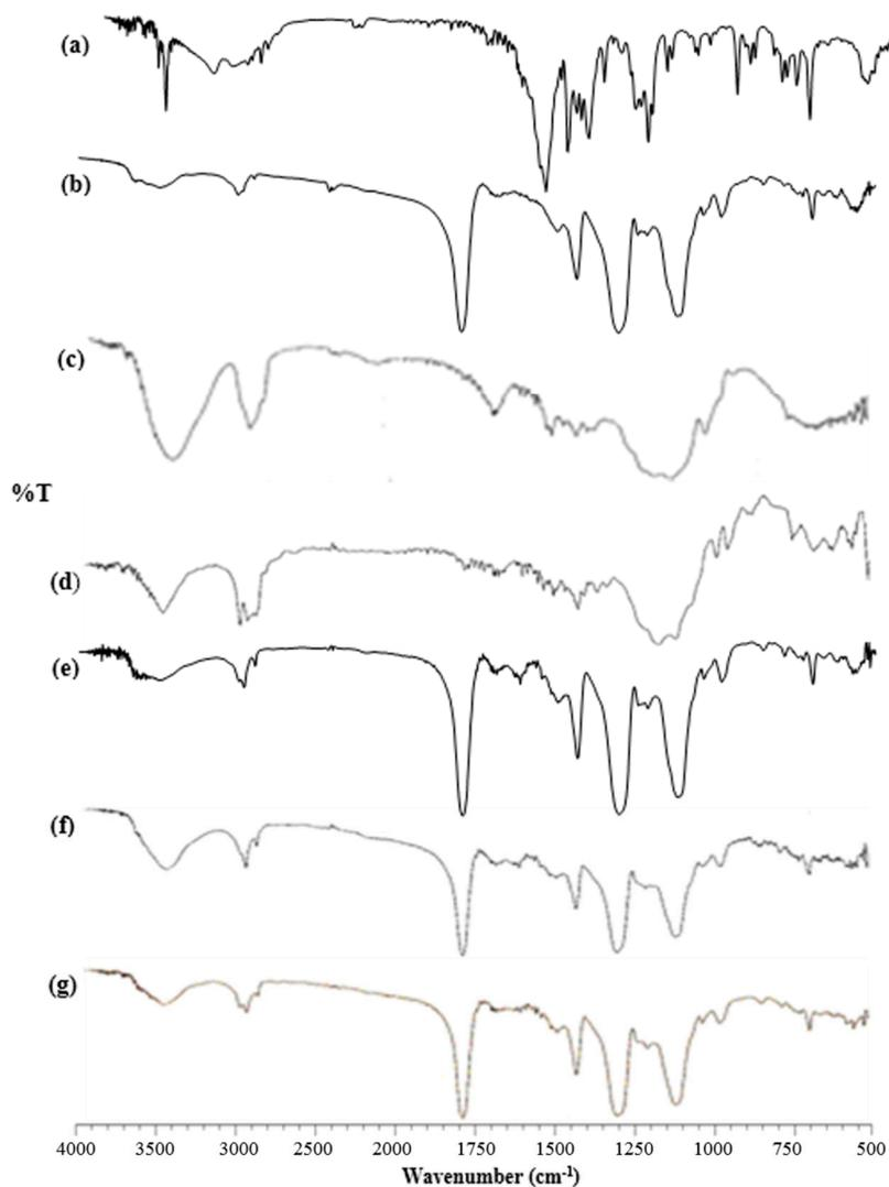
**Figure 4.** IR spectra of: fenoprofen calcium dihydrate (a); TA- $\beta$ -CD (b); HPMC (c); EC (d); drug-TA- $\beta$ -CD complex 1:3 (e); HPMC/drug complex (f); EC/drug complex (g). ( $\nu$  C–O–C asymmetric ether stretching), 933–696  $\text{cm}^{-1}$  ( $\nu$  primarily aromatic out of plane bending) [49]. TA- $\beta$ -CD exhibited a very strong absorption band at 1751  $\text{cm}^{-1}$ , due to C=O vibration of the acetyl (OCOCH<sub>3</sub>) groups [50].
