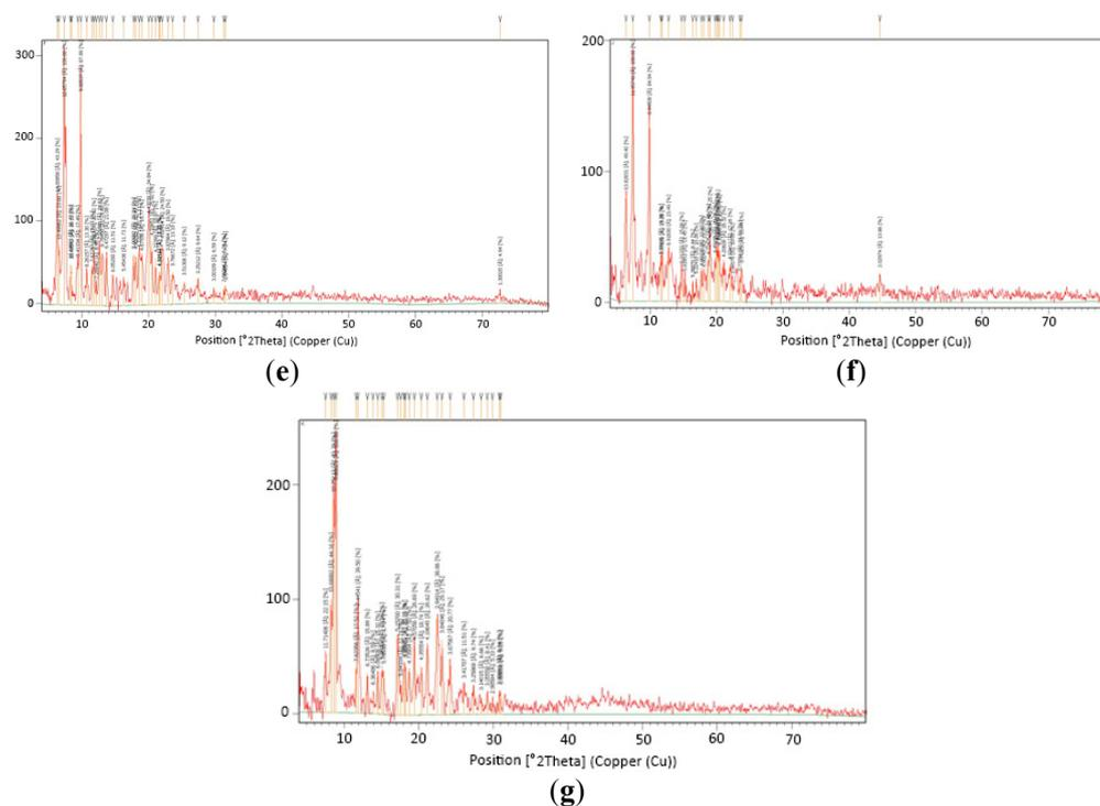
**Figure 5.** X-ray diffraction patterns of: fenopropfen calcium dihydrate (a); TA- $\beta$ -CD (b); HPMC (c); EC (d); drug-TA- $\beta$ -CD complex 1:3 (e); HPMC/drug complex (f); EC/drug complex (g). Note: The red color in each graph is characteristic for each substance respectively as shown in the figure caption and the yellow color is just a mark to indicate the peaks position and heights.
