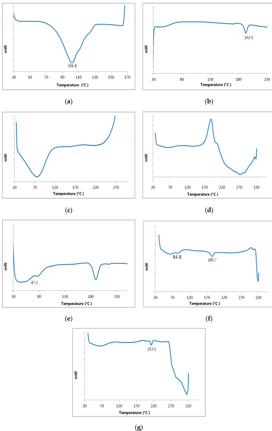
**Figure 3.** Differential scanning thermograms of: fenopropfen calcium dihydrate (a); TA-β-CD (b); HPMC (c); EC (d); drug- TA-β-CD complex 1:3 (e); HPMC/drug complex (f); EC/drug complex (g).
