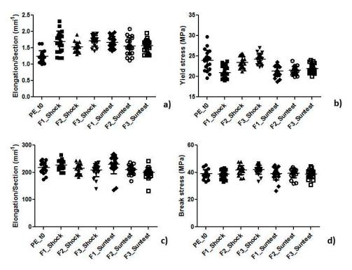
**Figure 2.** Trend of (**a**) yield strain; (**b**) yield stress; (**c**) break strain; and (**d**) break stress values obtained from all samples.
