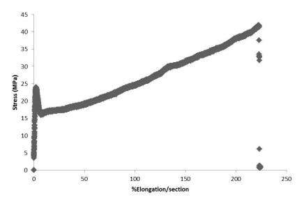
Figure 1. Example of a diagram obtained from the tensile test of the packaging.
