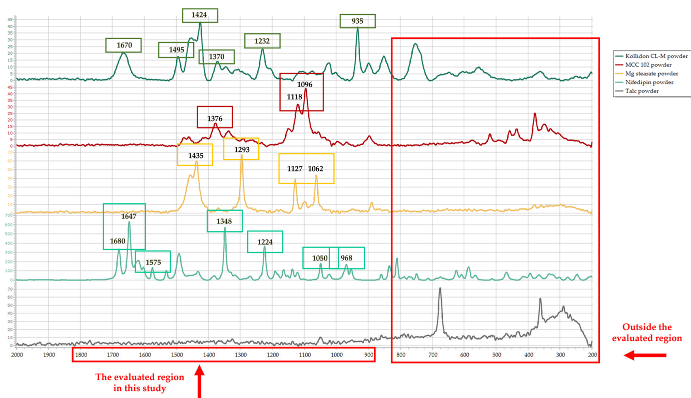
Figure 4. Raman spectra of pure HPMC, Kollidon ® CL-M, MCC 102, Mg stearate, nifedipine and talc powders, respectively.
