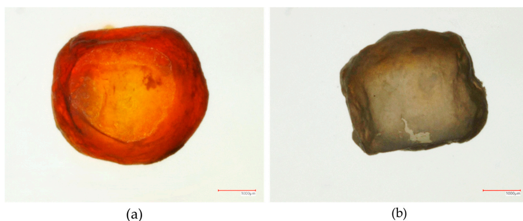
Figure 7. Illustration of the core during dissolution. (a) Before dissolution: The inert core with the drug layer distributed within the polymer shell, (b) After dissolution: The reconstituted inert core remaining within an intact polymer shell.
