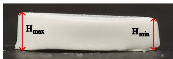
Figure 7. Representative side-view photograph of fixed SW-MT after 40 min of dissolution, illustrating post-dissolution height asymmetry and the locations of H_{\min} and H_{\max} .
