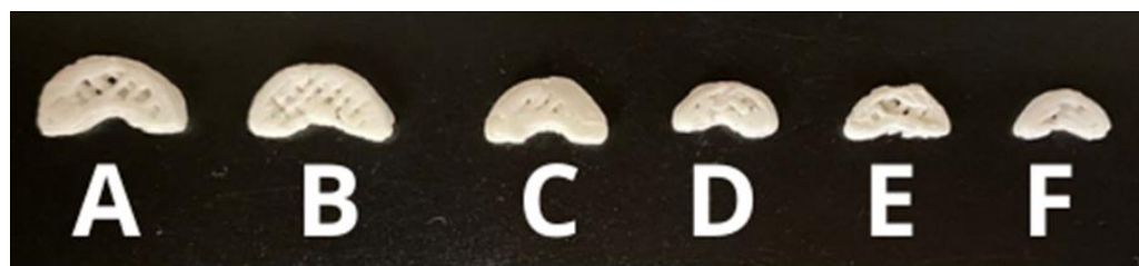
Figure 12. Printed with DOM-NC-3D of different sizes, A being the largest and F the smallest.
