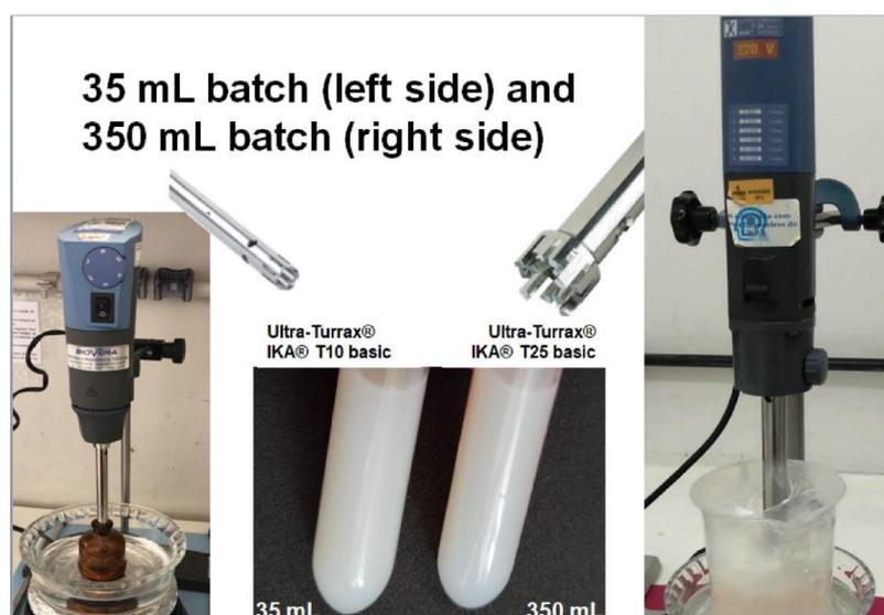
**Figure 5.** Preparation of 35 mL nanoemulsion batches under heat using a T10 basic Ultra-Turrax® IKA (left) and a process scale-up to 350 mL batches using a T25 basic Ultra-Turrax® IKA (right). The middle panel shows the disperser tools of each piece of equipment and the appearance of formulations.
