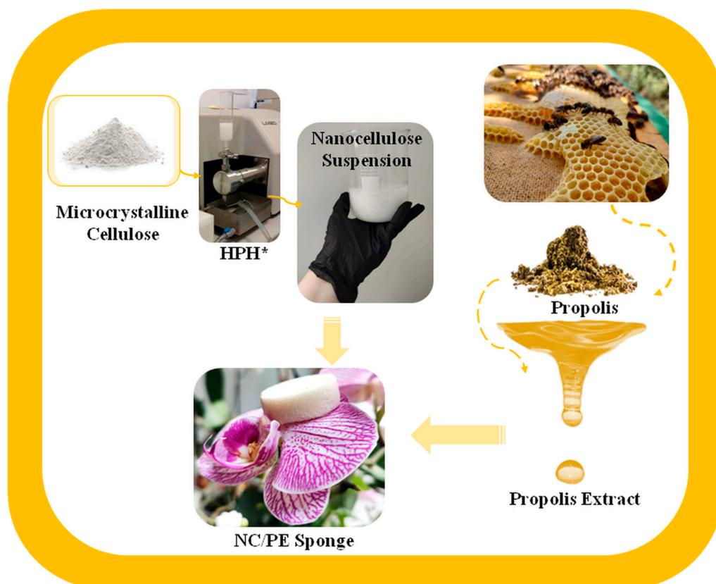
**Figure 1.** Schematic representation of the phases involved in obtaining the NC/PE sponges, where HPH\* represents high-pressure homogenization.
