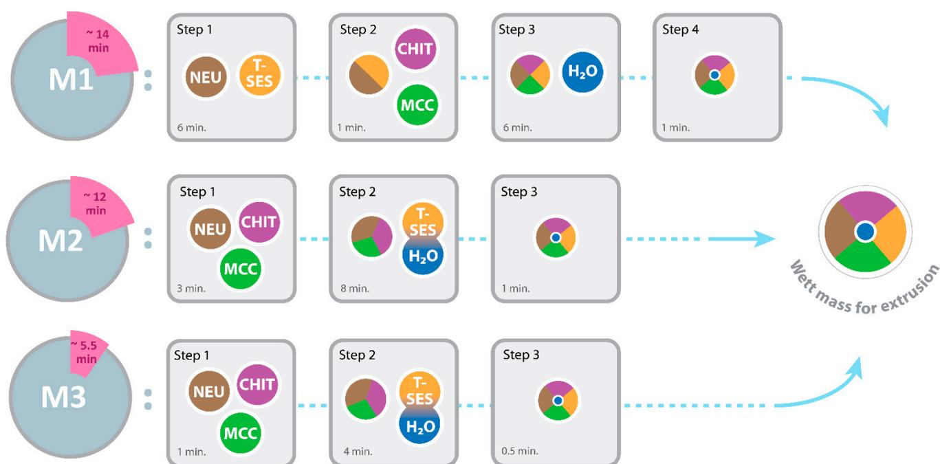
**Scheme 2.** Graphical representation and timeline of the three different preparation procedures (M1, M2, and M3) of uncoated pellet samples. The duration of individual steps, as well as the duration of the whole process (cumulative time), are presented.
