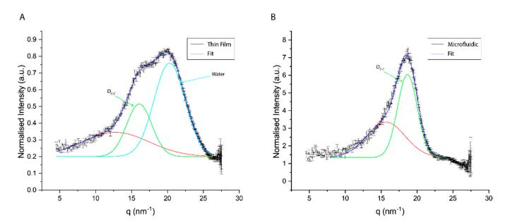
**Figure 8.** Fitting results of wide-angle scattering peak in both (**A**) MF and (**B**) TF samples. ( $D_{C-C}$ )—Chain-Chain distance. Red line for background.
