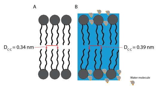
**Figure 13.** Schematic representation of the lipid structure in liposome mono-bilayer prepared via (**A**) microfluidics, (**B**) thin-film rehydration (blue square and stylized water molecules represent high hydration level). The inter-chain distance differences as well as the degree of disorder are exaggerated in the schematic to highlight the structural differences of both preparation methods.
