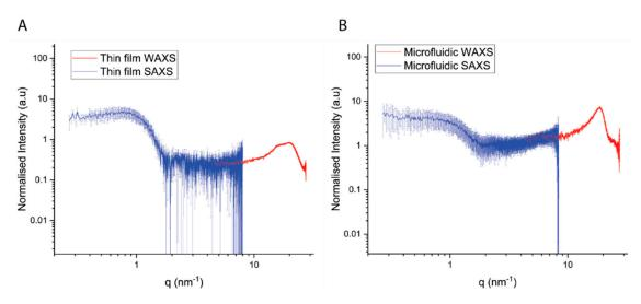
**Figure 7.** Normalized scattering intensity for lipid bilayer prepared via **(A)** TF, **(B)** MF. SAXS data are presented in blue, while WAXS data are in red.
