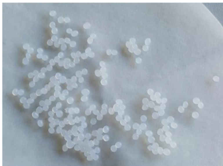
Figure 9. 2% HMW 80/1000 chitosan gel microcapsules formed when dropped from a distance of 10 cm.
