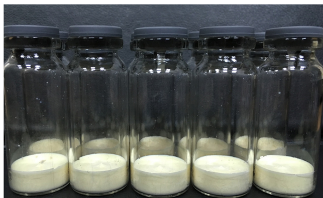
Figure 3. Typical freeze-dried cakes of Pz formulations with excipients in vials.
