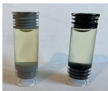
Figure 1. Example of the two sealing elastomeric gasket pieces (black colour right one and grey colour left part of the figure) located in the glass syringes.
