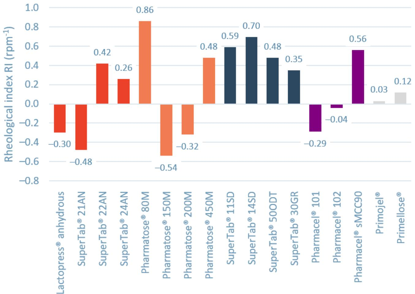
**Figure 3.** Rheological index (RI) values for the different materials. A positive rheological index indicates shear thickening behavior, while negative rheological index indicates shear thinning behavior. Different colours represent different types of materials.
