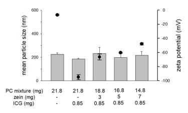
**Figure 2.** The effect of the zein-to-PC ratio on the mean particle size and the zeta potential of Z/PC-NP. The closed circle symbols indicate the zeta potential and the bars indicate the mean particle size.
