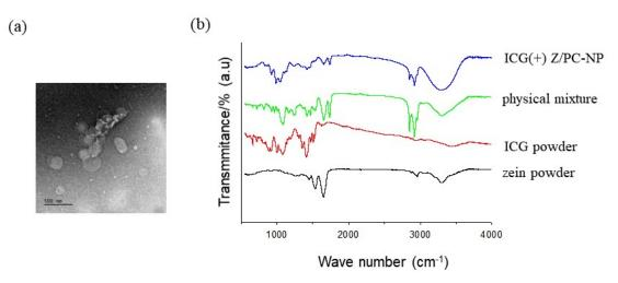
**Figure 1.** (a) A representative negative staining TEM image of ICG-encapsulated Z/PC-NP. Scale bar: 500 nm. (b) A FTIR spectrum of zein powder, ICG powder, physical mixture and ICG-encapsulated Z/PC-NP (ICG(+) Z/PC-NP). The Z/PC-NP was prepared from 14.8 mg of lipid (DMPC:CHOL mixture) and 7 mg of zein. The Z/PC-NP samples were freeze-dried before FTIR measurement.
