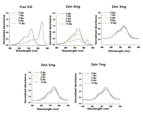
**Figure 3.** The effect of zein hybridization on the time-dependent formation of ICG J-aggregates. Changes in the absorbance spectrum of varying ICG formulations (0.85 mg/mL ICG concentration) were determined during incubation at room temperature. Free ICG solution was prepared in 5% D-glucose. The spectrum was obtained after sample dilution with 5% D-glucose and normalized by the 780 nm absorbance of each sample on the initial day.
