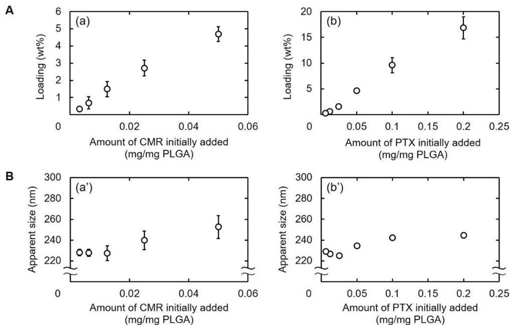
**Figure 2.** (A) Loading percentages of CMR (a) or PTX into PLGA-NS (b). (B) Apparent sizes of PVA<sub>200</sub>-PLGA-NS incorporating CMR (a') or PTX (b'). Various amounts of CMR or PTX were initially added for nanospheres preparation.
