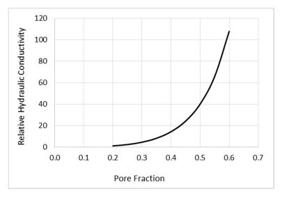
**Figure 3.** Relative increase of hydraulic conductivity, *K*, with increase in pore fraction,  $\varphi$ .
