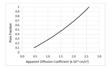
Figure 4. Estimation of pore fraction from measured apparent diffusion coefficient.
