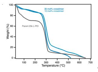
**Figure S2.** Thermal gravimetric analysis of crosslinked polymers. Cyclopropenium crosslinking of 25k L-PEI L-PEI provides enhanced stability below 300 °C. Crosslinking minimally changes thermal decomposition temperature. There is no change in thermal decomposition with increased crosslinking density.
