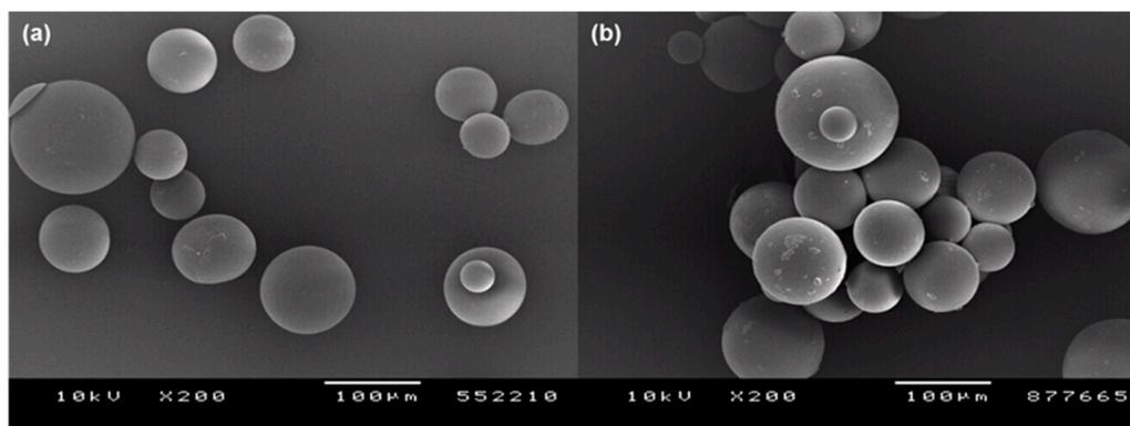
**Figure S2.** SEM micrographs of (a) blank PLGA microspheres and (b) those with the actual progesterone payload of 18.5%. The microspheres were prepared by the solvent evaporation process using methylene chloride. The size bar is 100  $\mu\text{m}$ .
