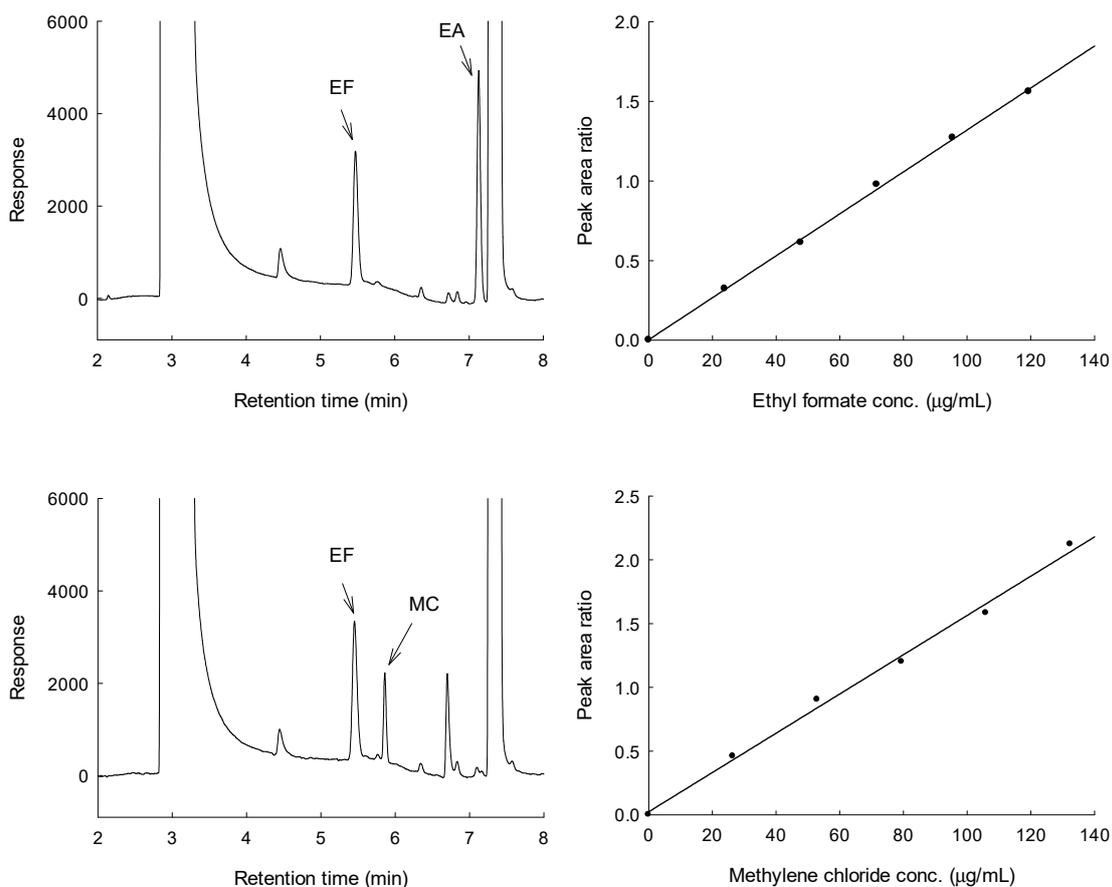
**Figure S3.** (Left) GC chromatograms of microsphere samples subjected to our GC analytical procedure. Arrows indicate the peaks of ethyl formate (EF), ethyl acetate (EA), and methylene chloride (MC). (Right) Standard calibration curves of the peak areas ratios vs. an analyte (ethyl formate or methylene chloride) concentration.
