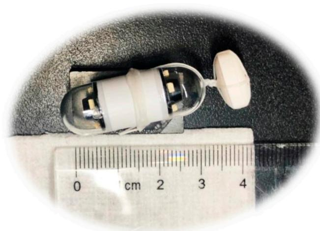
**Figure 1.** A dosage form is fixed in front of the camera capsule with a soft string (dental floss).
