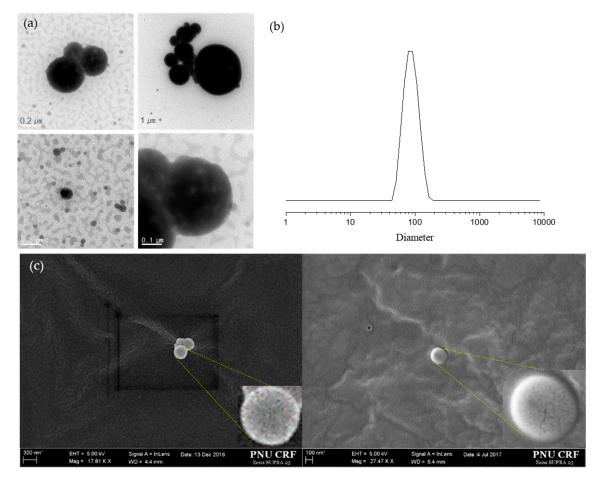
Figure 4. (a) TEM images, (b) DLS analysis, and (c) FE-SEM images of PFU nanoparticles.
