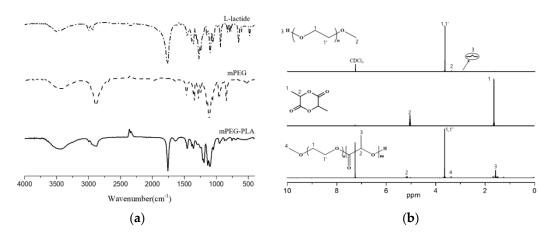
Figure 3. (a) FT-IR and (b) <sup>1</sup>H-NMR spectra of L-lactide, mPEG and mPEG-PLA.
