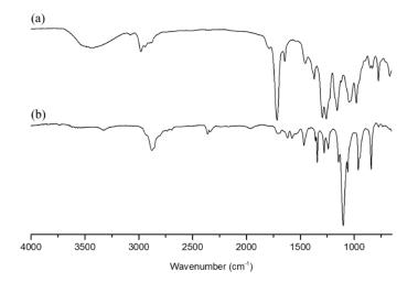
**Figure 1.** Fourier transform-infrared (FT-IR) spectra of (**a**) di-(2-hydroxypropyl fumarate) (DHPF) and (**b**) PFU.
