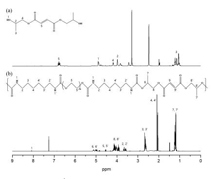
**Figure 2.** <sup>1</sup>H-NMR spectra of (**a**) DHPF and (**b**) PFU.
