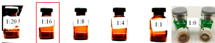
Figure S5. Physical appearance of lyophilized product of AMB-IONP with different weight ratios of sucrose. (Sucrose weight ratio of 16 and higher found to be optimum without any visible abnormalities of the cake).
