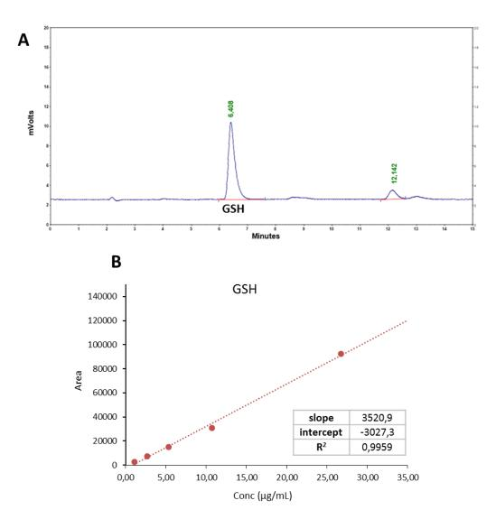
**Figure S2:** HPLC chromatograms of a standard GSH solution (Rt = 6.4 min), while the unreacted 1,4-Naphthoquinone (NPQ) is detected at Rt = 12.1 min (**A**); HPLC linearity: calibration plot, slope, y-intercept and determination coefficient of GSH (**B**)
