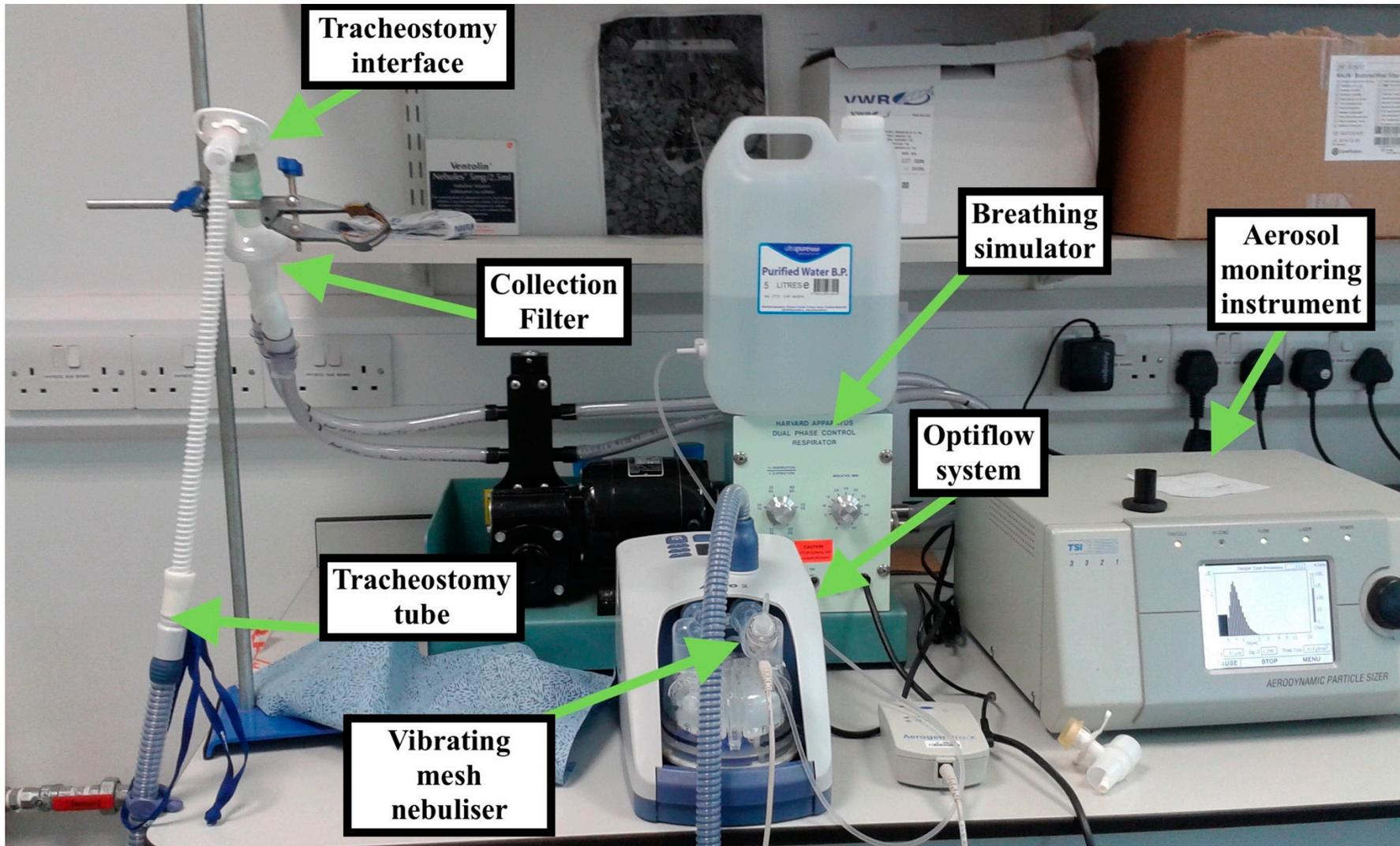
Figure S3. A photograph highlighting the physical setup for the adult and paediatric tracheostomy set up.
