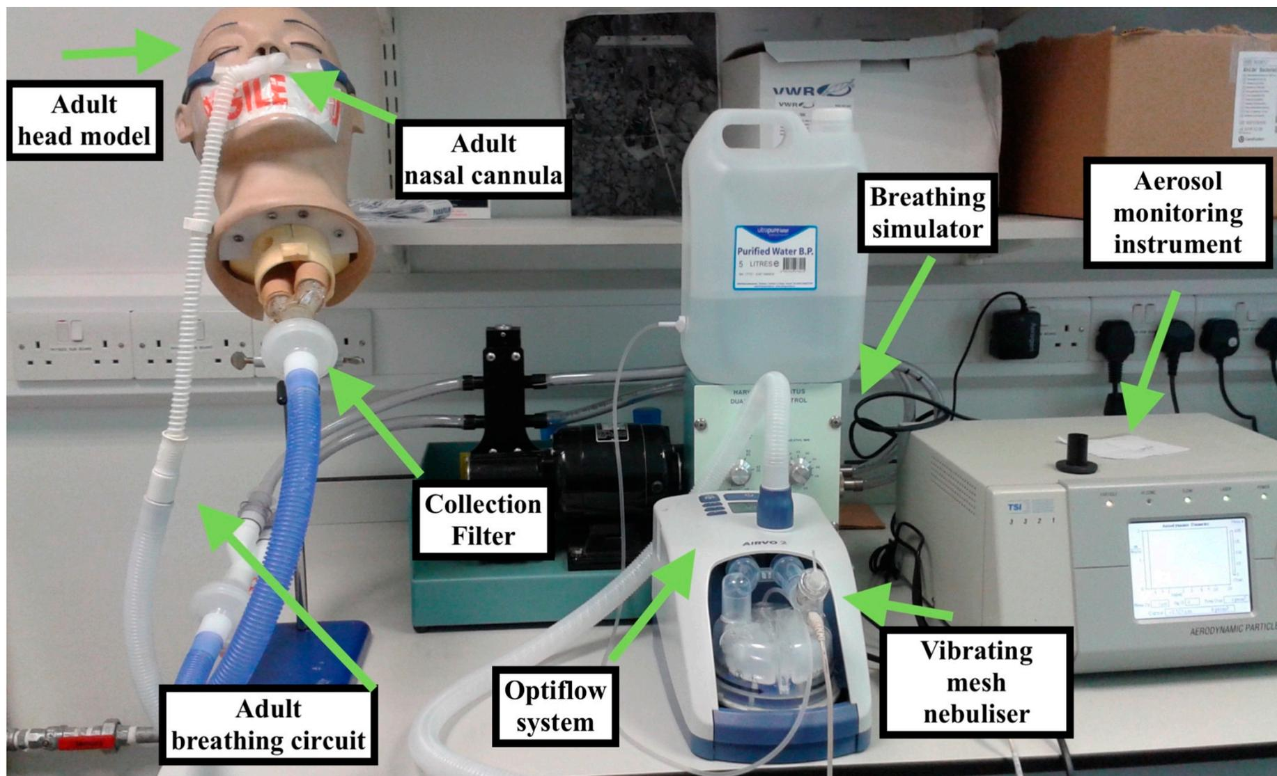
Figure S2. A photograph highlighting the physical setup for the adult nasal cannula set up.
