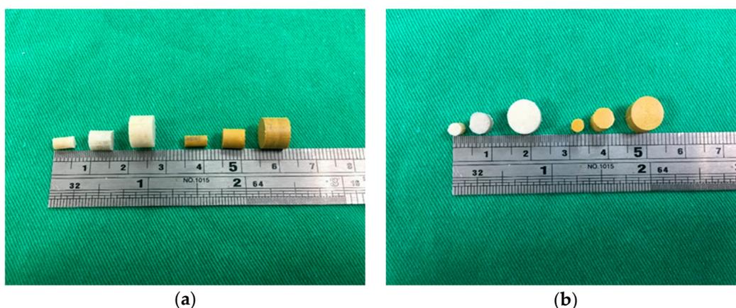
**Figure 3.** Photographs of the fabricated drug-loaded beads. The white cylindrical beads are fluconazole-impregnated Poly(*D,L*-lactide-co-glycolide) (PLGA) beads. The yellow cylindrical beads are amphotericin B-impregnated PLGA beads.
