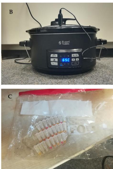
**Figure 2.** Loop-mediated isothermal amplification (LAMP) assay without a thermocycler. (A) Comparison of RT-PCR vs. the LAMP assay performed in a household sous-vide cooking unit. (B) Picture of the sous-vide cooking unit during testing, and (C) of the samples after completion of the assay.
