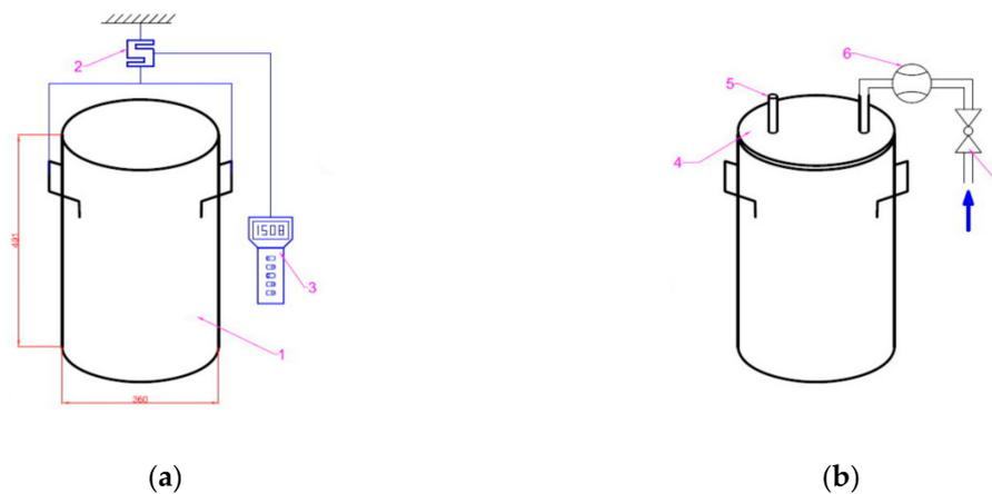
**Figure 1.** Scheme of the measurement setups: (a) for bulk density, (b) for the conversion factor: 1—measuring container, 2—load cell, 3—recorder, 4—lid, 5—air escape, 6—electronic flow meter, 7—valve.
