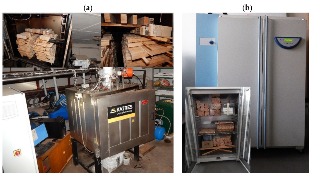
Figure 2. The photograph of the thermal chamber used for the treatment including the arrangement of the samples inside (a) and the photograph of the conditioning chamber used for the conditioning after heat treatment including the arrangement of the samples inside (b).
