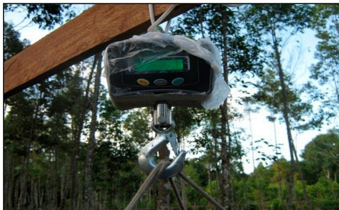
**Figure A5.** Digital scale for measuring the fresh mass of the mass harvested in the rosewood plantations.
