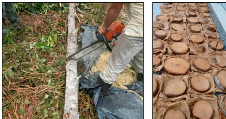
**Figure A6.** Collecting the wood discs at 0, 50, and 100% of the height of the trunk for calculate dry mass; and collecting the sawdust to calculate the mass of the tree.
