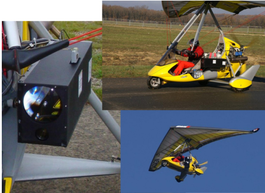
Figure 1. ULICE (Ultraviolet Lidar for Canopy Experiment) onboard an ULA (Ultra-Light Aircraft). The lidar optical head is shown on the left picture. The top right picture shows a global view of the lidar embedded on the ULA. The bottom right picture shows the lidar in flight during the experiment, with the optical head pointing downward.
