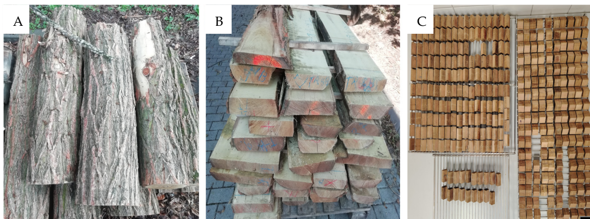
Figure 2. A R. pseudoacacia logs (A), boards (B), and specimens used for density, shrinkage, and swelling tests (C).
