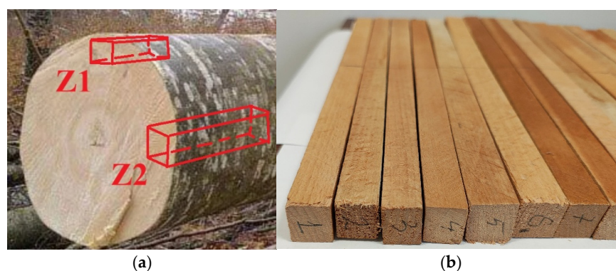
Figure 2. (a) Zones of the log from which the specimens used in the experimental program were extracted; (b) specimens prepared for testing.
