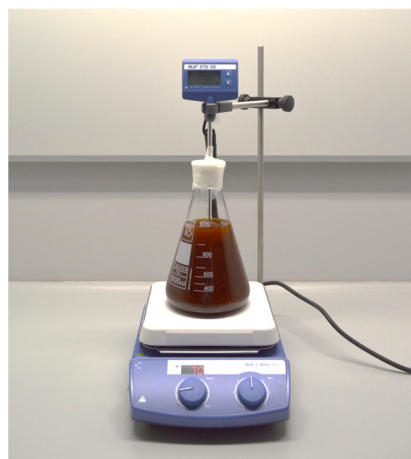
Figure 2. Extraction using a heated magnetic stirrer with temperature control (photo: Klarić, M.).
