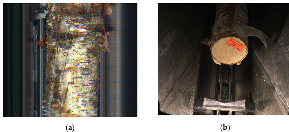
Figure 2. Examples of the visual data of a birch veneer log. (a) A part of the side-surface image obtained with a line-scan camera. (b) An end-face image obtained with an area-scan camera.
