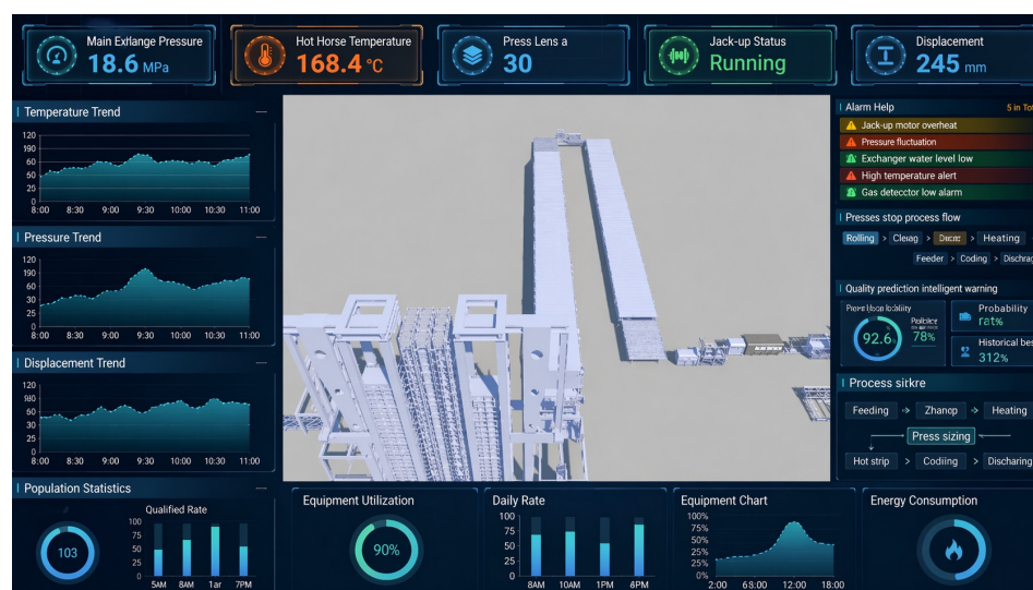
Figure 15. Digital Twin Monitoring Interface for the Hot-Pressing Process of Bamboo-based fiber composite material.
