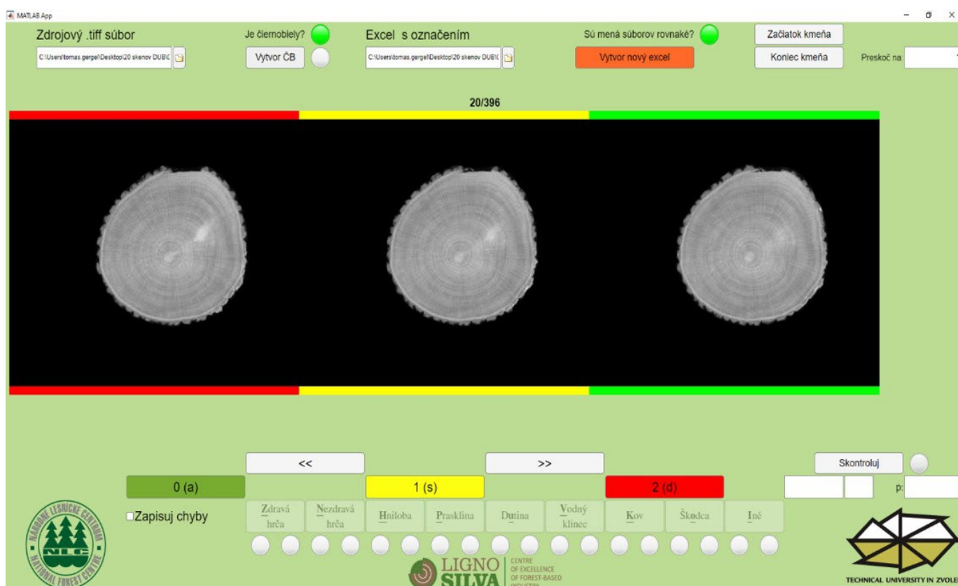
Figure 2. Application interface for simplified annotation of CT images for defect presence or absence.
