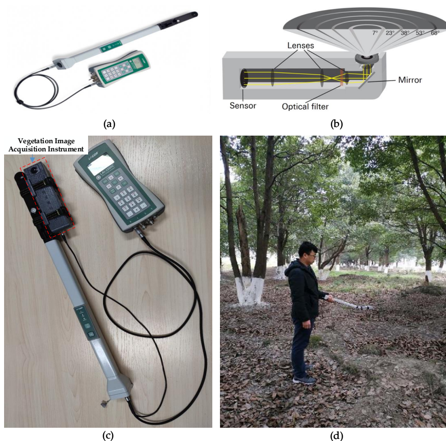
Figure 2. Experimental data collection. (a) LAI-2200C; (b) LAI-2200C measurement principle; (c) Experimental equipment connection diagram; (d) Experimental site map.
