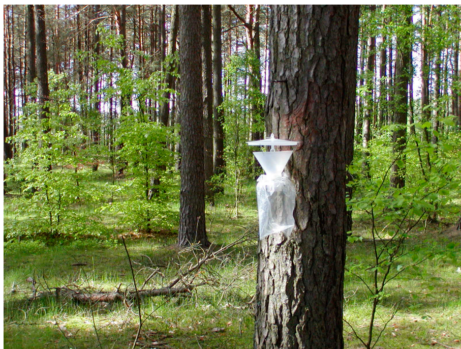
Figure 2. IBL-1 type pheromone trap in the field (Chemipan R&D Laboratories, Warsaw, Poland).
